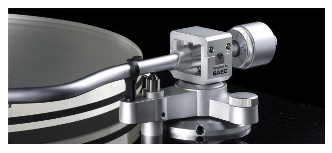
base can be adjusted. The Vertical Tracking Angle (VTA) can be adjusted in a 6mm range and optimized for cartridges of various heights. The tone arm geometry adheres to the Baerwald alignment recommended by the IEC.
