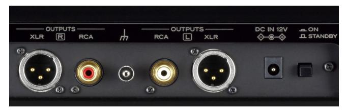
In addition to ordinary RCA connectors, XLR connectors are also available for analog output. A variety of commercially available cables can be used to connect with a PE-505 or other external phono equalizer that supports balanced XLR input.
